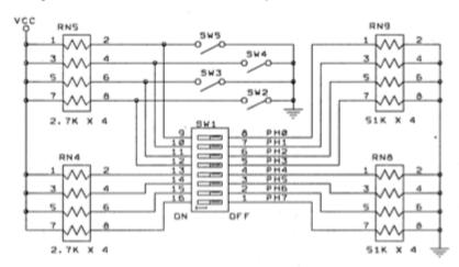
The DIP switch, SW1 should have all switches in their ON position. Then when the push buttons are not depressed, there is a 2.7K resistor to VCC and a 51K resistor to ground. The Port H pins will be at roughly 4.75 volts which will insure a high logic level. When a pushbutton is depressed the corresponding Port H pin voltage will drop to 0 volts, a low logic level. PH3 through PH0 are used for SW2 through SW5 respectively.
