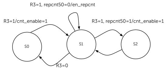
The state machine is intended to run at the 100 MHz clock rate. This can actually be implemented with two states, but three makes it a bit more interesting.
